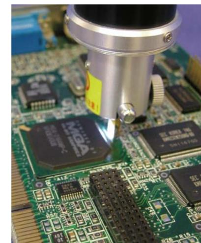
**QFP, Assembly Parts Inspection**
