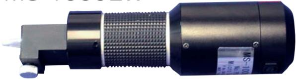
This model is fit for inspecting the BGA and QFP from a wide angle. You can also use it to view the interior section of a BGA package using the backlight system. Magnification: x70 on 14inch TV
